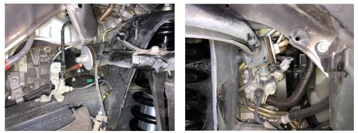
H. Carefully remove the UCA bolt. The UCA can now be removed. If still in good condition, save the UCA bolt and flanged nut as they will be reused. Otherwise, replace UCA bolt/nut. The OE washer can be discarded.
