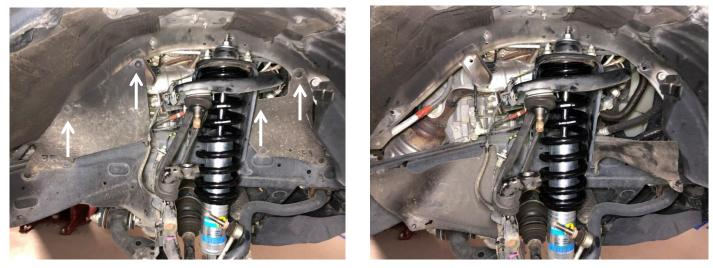
G. Using two 19mm wrenches, remove the nut and washer securing the UCA bolt.
