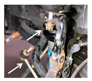
E. Using a ball joint puller, separate the spindle from the ball joint stem. Be careful to avoid tension on the brake line and ABS line.
