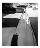
( **B** ) Use a small flat screwdriver and remove the plastic cap in the front ditch molding on either side of the sun roof to expose the threaded mounting points.
