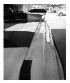
( **B** ) Use a small flat screwdriver and remove the plastic cap in the front ditch molding on either side of the sun roof to expose the threaded mounting points.
