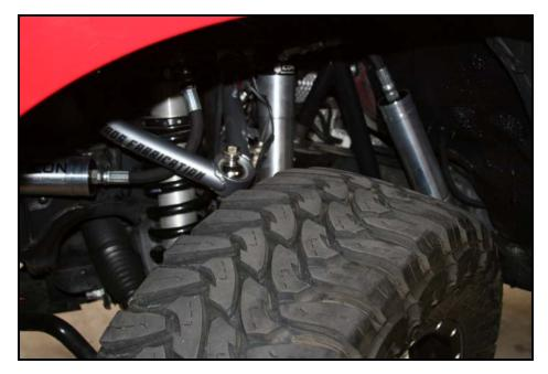
**Step 12:** After welding we recommend that you spray paint as much of the hoop and frame as possible before re-installing the secondary shocks.
