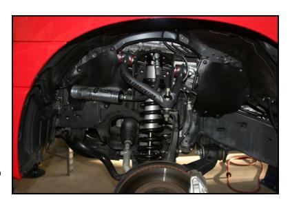
Step 5: Trace along the top of the hoops on the factory inner wheel apron. (Trimming the sheet metal is necessary to clearance the hoop. (Make sure to look inside the engine compartment while cutting). Check clearance on any stock components. It is recommended to cut under the marks you made, and then trim as needed checking hoop clearance at the same time. (See photo)
