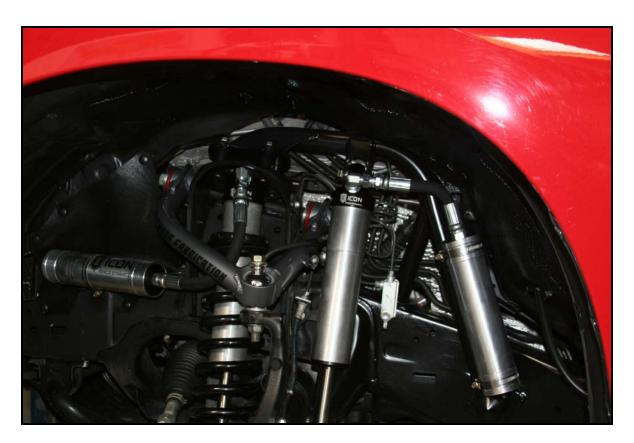
Step 14: Install the shocks on both sides with the supplied hardware and charge to manufactures recommended PSI.
