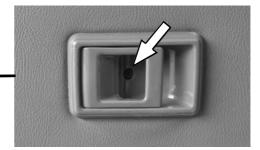
( **B** ) Pull the latch from the door card. Once the latch if free, the door card can be loosened and removed by gently pulling on it and feeding the latch back through the cut-out inside.
