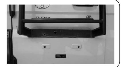
( **F** ) Fit the light removed in Step 2C back into position. The bottom of the Ladder will now be sitting between the light and the vehicle's door and is secured in position by the light. You may require a friend to apply weight to the Ladder in order to line the mounting holes up and refit the light.
