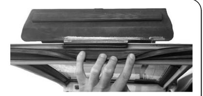
(**E**) Line up the mounting holes in the bottom of the Ladder with the light's mounting holes in the vehicle's door.
