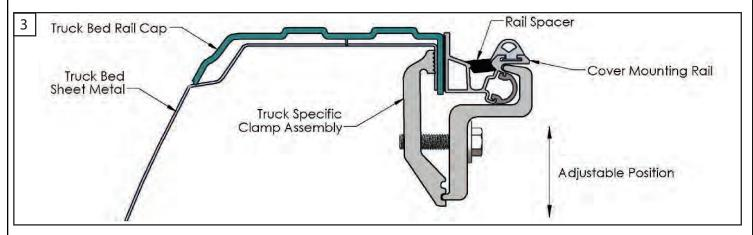
4. Tighten the clamps using a 1/2" socket.
