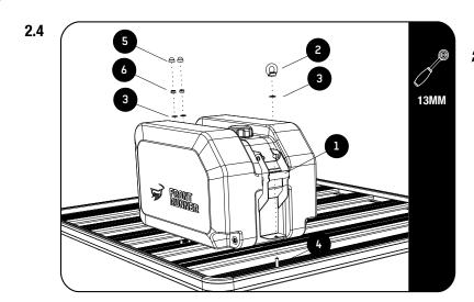
Place the Water Tank with Tank Strap onto the Rack as shown, lining up the holes in the Tank Strap (Item 1) with the Hex Bolts inserted in Step 2.2 and 2.3. Ensure that the Tank is sitting centered on the T-Slot Beading and secure the Tank Strap to the Rack using the M8 Eye Nut, M8 Flat Washer and M8 Nyloc Nuts (Items 2, 3 & 6) as shown.
