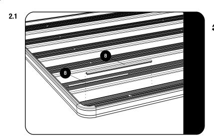
Choose to mount your 45L Water Tank (not supplied on either the front or back of the Slimline II. The Tank must be positioned using either the front or rear slat.
