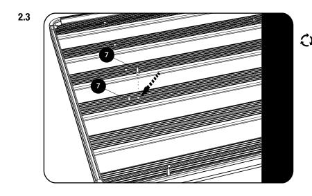
Slide the two M8 x 20 Hex Bolts (Item 7) into the T-Slot on the third Slat from the back of your Rack as shown.
