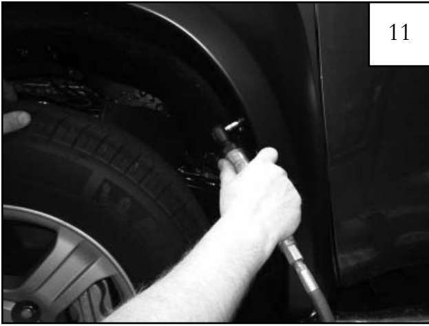
Start Screw (SW1-0036) through the one lower rear hole in flare and into factory hole in lower rear of wheel well.
