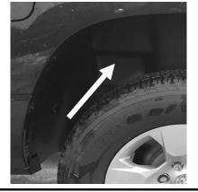
NOTE: <u>Make sure</u> the hole on the plastic moulding bracket behind the wheel well liner is aligned with the holes on the sheet metal and wheel well liner
