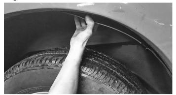
**7.** Locate the pre-drilled hole on the plastic liner located towards the front of the truck then install the screw saved on step 1.
