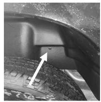
**8.** Tighten the screws that were loosened in step 2
