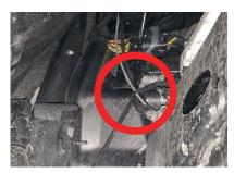
8. Route the wire over the top of the frame rail and secure the harness wire to another wire or fixed point using zip ties. Then route the harness wire along the frame rail toward the rear wheel well and secure using zip ties.
