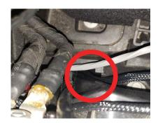
7. Route the harness output wire through the small opening in the engine bay to the passenger wheel well, located between the battery and the passenger fender.
