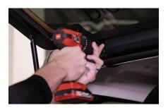
1. Open the hatch and locate the four 10mm bolts holding the back glass brackets in place. Remove two of the 10mm bolts from one side of the vehicle. Be sure to only remove two bolts at a time to provide enough support to the back glass.
