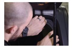
4. Open the hatch and route the wiring behind the glass and tuck it into the channel behind the weather stripping as shown in the picture to the left. You may also choose to use the included adhesive wire clips to secure the wiring in place.
