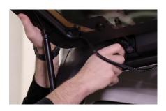
2. Using one hand to support the back glass, set the bracket into place. Then reinstall the 10mm bolts. Repeat for the other side of the vehicle.
