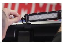
3. Close the hatch and mount your light bar to the brackets using the included 10mm bolts.
