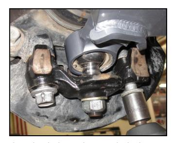
**17.** Once all steps have been completed, go back through every bolt that was loosened and make sure that it has been re tightened and/or torqued to proper spec.
