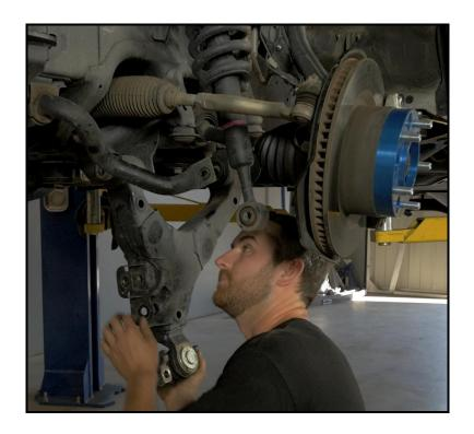
**7.**After removing the lower control arm, remove the cotter pin and ball joint nut using a 24mm wrench or socket, then use a hammer to shock the stock ball joint cradle and separate it from the ball joint. If this does not work, you can use a pickle fork to remove the cradle.
