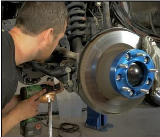
**4.**Loosen (do not remove) the two cam bolts that connect the lower control arm to the vehicle using a 24mm wrench or socket.
