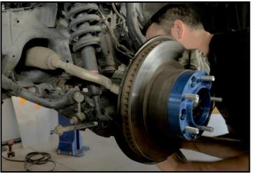
**3.**Remove the bolt that connects the sway bar link to the stock lower control arm as well as the nut that secures the link to the sway bar using a 19mm wrench or socket.
