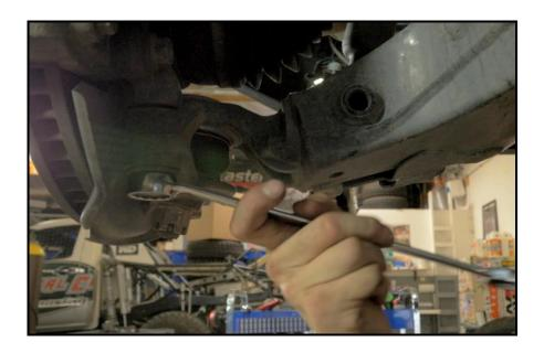
**6.**Let the lower control arm pivot down into a vertical position, then remove the two bolts that hold the control arm to the frame, and remove the stock lower control arm from the vehicle.
