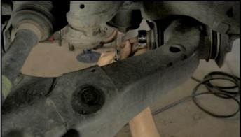
**5.**Remove the two bolts that hold the ball joint cradle to the steering knuckle using a 22mm wrench or socket.
