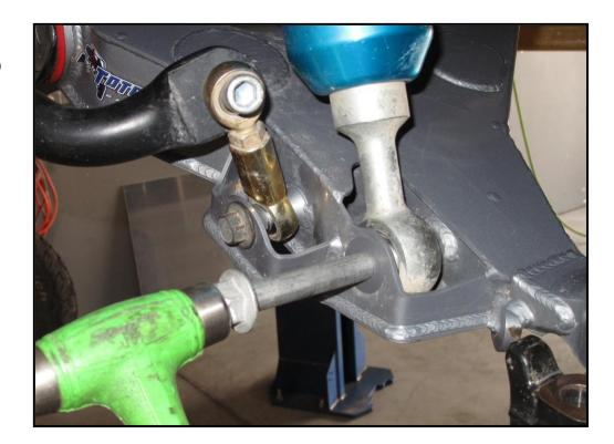
**16.** Lower the spindle onto the ball-joint cradle and install the stock bolts.
