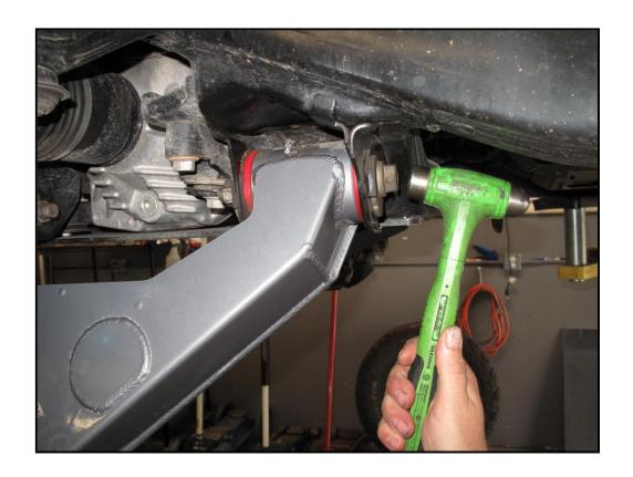
12.Install the short misalignment in the top of the uniball, the large misalignment into the bottom of the uniball (tapered side down), slide the ball joint cradle onto the tapered misalignment, then slide the bolt from the top through all of the pieces then install the washer and tighten the nut using a 5/8" Allen wrench and 1 1/8" wrench or socket (110ft/lbs).
