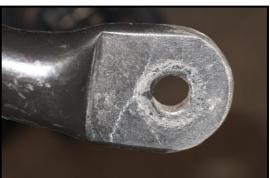
10.Install the supplied bushings, inner sleeves, and zerk fittings into the new lower control arm, then install the new arm on the vehicle (it may take the use of a dead blow hammer to get the arm into the frame pockets).
