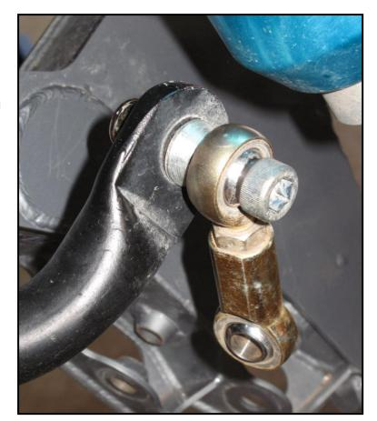
14. Next swing the control arm into the horizontal position and install the other end of the heim into the lower control arm using the flange head bolt and a 21mm wrench to hold the nut inside the arm.
