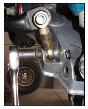
15. Move the control arm up slightly and install and tighten the shock bolt.
