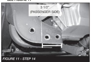
Locate the factory front lower control arm pockets. Grind ¼" section from both Corners of the pockets.
