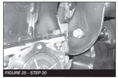
21. Locate and install FT20610BK front crossmember into the factory lower control arm pockets using the stock hardware. Leave loose. (CHECK THE CLEARANCE OF THE DIFF TO CROSSMEMBER WHERE IT WAS SANDED DOWN IN STEP #18 FOR ADAQUATE CLEARANCE TO THE FRAME AND CROSSMEMBER). **SEE FIGURES 26-27**
