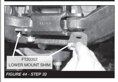
LOOKING TOWARDS GROUND, TURN ONLY IN COUNTER CLOCKWISE DIRECTION AND ROTATE AS NECESSARY
