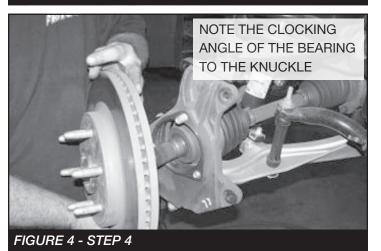
5. Remove the upper and lower ball joint nuts. Disconnect the upper and lower ball joints from the steering knuckle by striking the knuckle with a large hammer next to each ball joint on the knuckle to dislodge the ball joints. Use care not to hit the ball joints when removing. Save nuts
