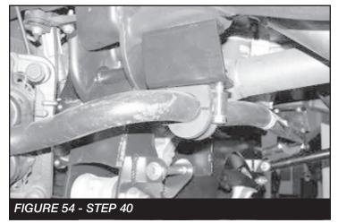
41. Locate FT20602 Sway Bar Mounts and the supplied 18mm x 50mm hardware. Position the Sway Bar Mount so that it is on the bottom of the sway bar with the SHORTER side of the mount against the stop plate end of the mount. Attach with the 18mm hardware and torque to 110 ft-lbs. Locate the factory sway bar end links and attach to the new mount and the lower control arm. (NOTE - SOME PICK UP TRUCKS MAY BE EQUIPPED WITH SUV STYLE SWAY BAR). SEE FIGURE 55
