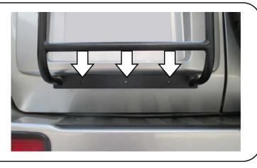
(G) Position the Ladder back onto the vehicle and secure in place using the fasteners supplied as in Step 2F. Place a M6 Nut Cap (Item 1) over the head of each bolt once fully tightened.
