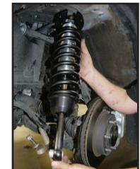
**8**. Connect the shock to the lower control arm: The lower shock mount has (1) long and (1) short spacer [Torque to factory spec]. Make sure the long spacer is toward the front of the vehicle as this will position the shock further toward the rear of the A-arm to ensure adequate sway bar clearance. Install the factory lower shock bolt.
