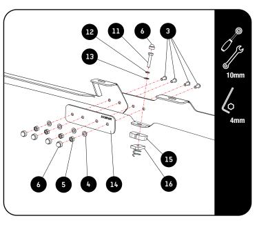
Join the two halves of the foot rails with the supplied splice plate (Item 14). Fasten as shown with items 5, 4 and 3.
