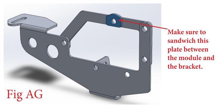
33. IF YOU DO NOT PLAN TO RELOCATE YOUR ADAPTIVE CRUISE CONTROL MODULE, PLEASE SKIP THIS STEP. Mount your adaptive cruise control module/bracket assembly to the intercooler. Use a 13mm Socket & Wrench along with the supplied M8 Bolts (x2), M8 Washers (x3), and M8 Lock Nut (x1). First, position the adaptive cruise module so that it is completely straight with the intercooler. Then, point it slightly towards the sky and tighten both mounting bolts. (Fig AH)
