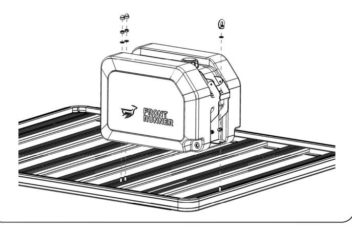
( **D** ) The Water Tank may be taken off the Rack by removing the Plastic Cap (Item9), loosening the M8 Eyenut and lifting the Tank Strap up and over as shown.
