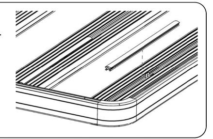
( **B** ) Using a 4mm Hex Key, loosen and remove the Corner of the Rack as shown.
