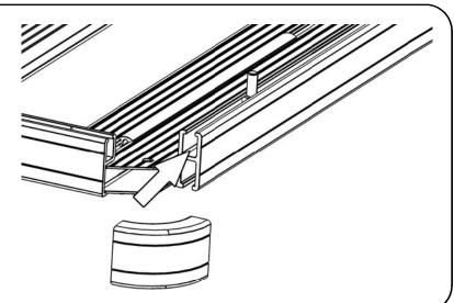
Slide the two M8 x20 Hex Bolts (Item 8) into the T-slot on the third Slat from the rear of your Rack through the Machined Slot as indicated by the arrows.
