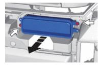
2. Using a Phillips screwdriver, remove the two screws securing the factory fog light to the front bumper. Then remove the factory fog light from the vehicle, and unplug the factory fog light connector.
