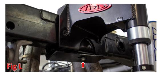
2. Set the Bump Stop Cross Member in place. Secure it by loosely installing the supplied 3/8 x 1 1/2" Bolts (x4) and 3/8" Washers (x4). (Fig M)
