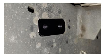
O. Using the other two M8x1.25 Flat Head Cap Screws, apply non-permanent thread locker and fasten Reservoir Bracket assembly to the Reservoir Slot Bracket as shown below.
