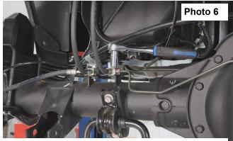
Remove the brake lines from the axle.
