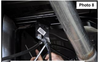
Install the emergency brake bracket.
