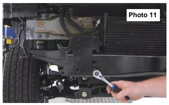
Remove the front bumper mounting plates.
