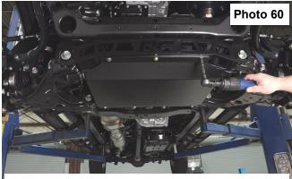
Install the new supplied skid plate.
