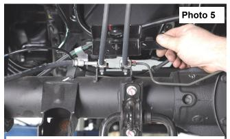
Remove the brake line shield.
