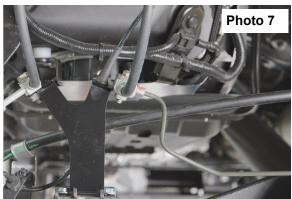
Install the brake line relocation bracket.
