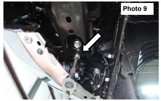
Remove the lower bumper mounting bolts.
