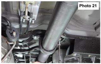
Tighten carrier bearing bracket.
