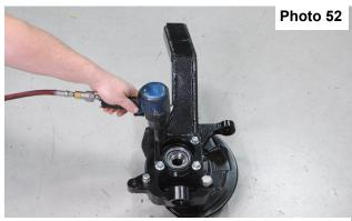
Install bearing assembly into lifted knuckle.
