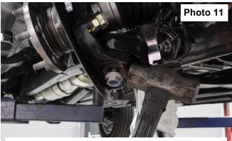
Strike knuckle to release taper on lower ball joint.
