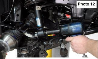
Remove the lower strut hardware.
