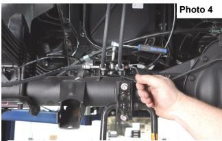
Remove the brake line shield.
