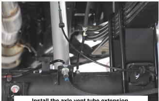
Install the axle vent tube extension.
