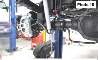
Install the shock in the lower mount.
