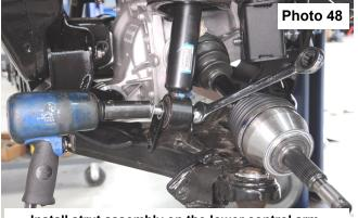
Install strut assembly on the lower control arm.
