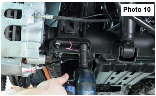
Remove the factory u bolts and hardware.
