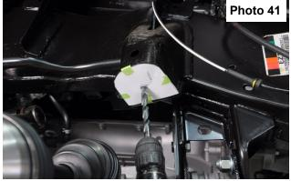
Drill using a 13/32" drill.
