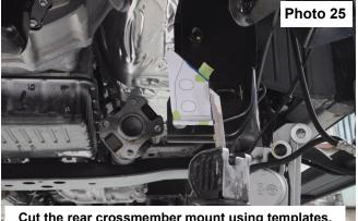
Cut the rear crossmember mount using templates.
