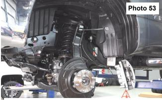
Install assembled knuckle onto vehicle.
