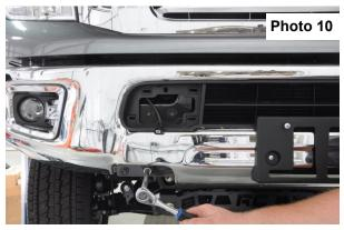
Remove the front bumper mounting bolts.
