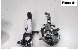
Remove steering stops from factory knuckle.
