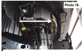
Drill or slot hole to front of truck.
