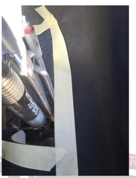
Starting on the rear line at the point where the bed floor and the wheel well connect, measure back 1", connect this dot to the pinch weld seam. Measure upwards along the cutout 2".
