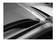
(  ${f C}$  ) Using a 10 mm wrench, loosen the six bolts each side securing the rails to the vehicle.
