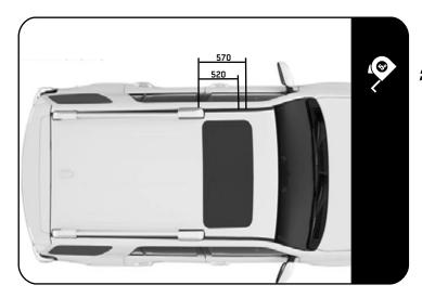
With the factory rails removed, use the center of the existing front hole of the roof rail, mark out the dimension as shown on the ditch molding. Do this on the left and right side.
