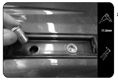
Drill the pilot holes to 11.5mm and secure two rivnuts (item 9) in the holes by using a rivnut setter.
