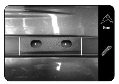
Place the spacer (item 10) over the marks you have made. Mark the outsides of the spacer.
