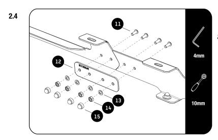
Assemble the front and rear foot rail (items 1 and 2) with the joiner plate (item 12) with the fasteners shown.
