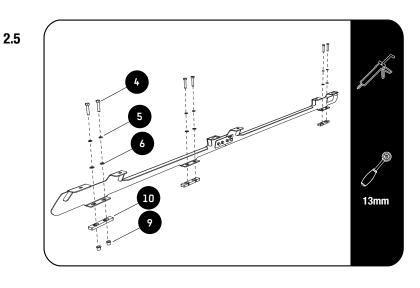
Place a bead of sealant in and over each hole in the roof, then place a spacer (item 10) over each hole.
