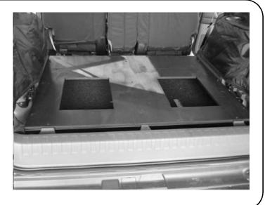
(E) Place the Left and Right Top Decks (Items 2 & 3) onto the Bottom Deck, lining up the front edges (Passenger seats side) of the Top Decks with the front edge (Passenger seats side) of the Bottom Deck. once happy with the positioning of the Top Decks, secure the Top Decks to the Bottom Deck using the Wood Screws (Item 11) supplied. Below is the suggested pattern to follow when securing the decks.
