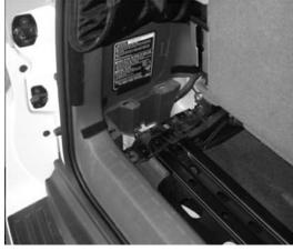
$(\ {\bf F}\ )$  Using a panel tool, remove the rear plastic trim as shown.
