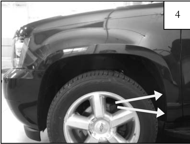
Using a 7mm socket, remove two factory screws. Retain screws for later use.
