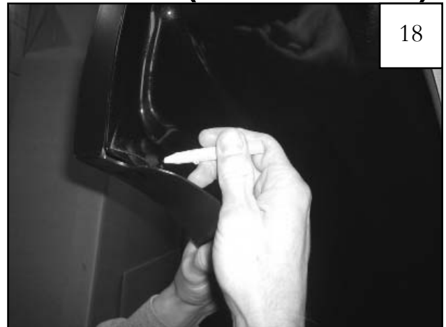
Using a grease pencil, mark four hole locations on the inside of the door by aligning the marks with the holes in flare.
