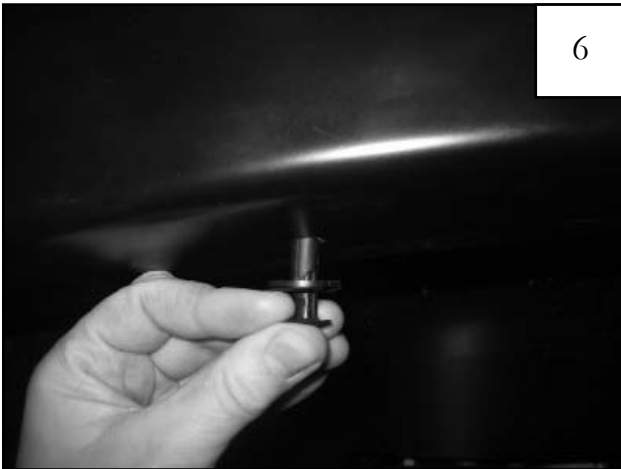
Install two supplied Retainers (RV1-P006).
