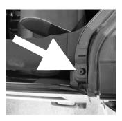
(D) The Aluminum Tracks ship with the Rubber Linings loosely fitted in place. There are two quick steps to prep the Liners and Tracks. Start by removing the paper backing to expose the glue. Carefully center the holes in the Liner with the holes in the Track and press the Liner into place. Grab your scissors and trim the Liner at the end of each Track so it doesn't overhang. You can cut an angle with the slant of the track, or make a straight cut. You might want to practice first.
