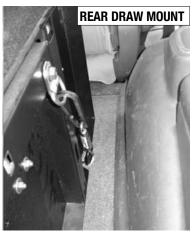
( C ) Fit the four Deck Side Skirt Support Brackets to the side of the Draw System (Two left, two right).
