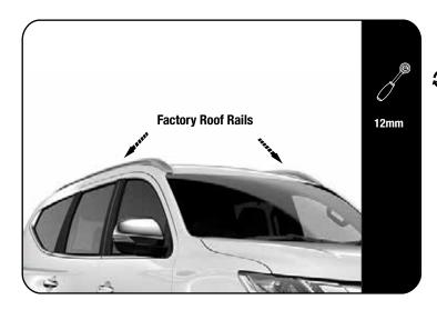
Before you start with the fitment of the foot rails, you need to remove the factory roof rails. Do this by unclipping and removing the front and rear end-caps of the roof rail. In the middle of the roof rail you will see a small cover plate, this will also need to be removed. Now loosen the two bolts in front, one bolt in the middle and 3 bolts at the rear of the roof rail.
