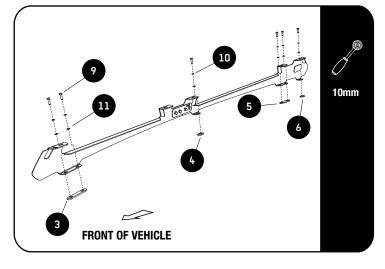
Place a bead of sealant in and over each hole in the roof, then place the spacers (items 3, 4, 5 & 6) over front, middle and two rear holes as shown.
