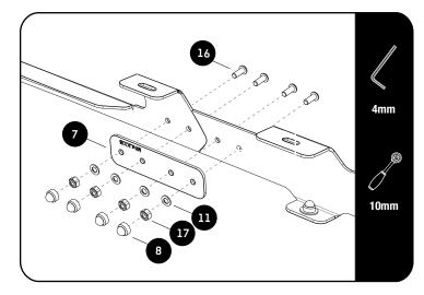
Assemble the front and rear foot rail (items 1 and 2) with the joiner plate (item 7) and fasteners (items 16, 11, 17 & 8) as shown.
