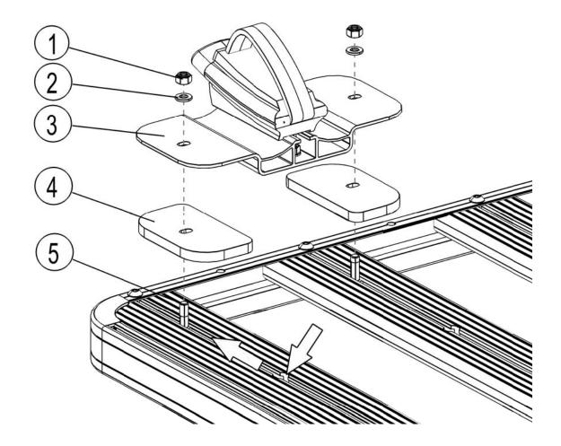
(A) Insert a M8 x 25 Hex Bolt (Item 5) into each of the required slats using the Machined Slot as indicated by the arrow.
