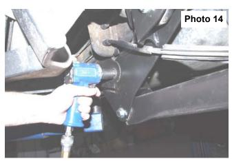
21. Tighten the new 9/16" hardware using a 13/16" socket. Torque to 95 ft-lbs. See Photo 15.
