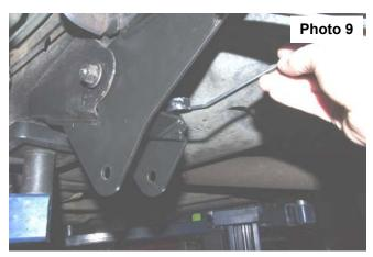
16. Install the supplied 14mm x 40mm bolt, flat washer, and lock washer (1287BAG1) into the flag nut, through the bottom of the control arm drop bracket and the factory lower control arm mount. **Do Not Tighten. See Photo 10.**
