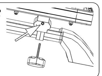
(B) To complete your installation, center the Rack from left to right using a tape measure. Ensure that the Strap-on Feet are sitting all the way in on the Adapter Plates. Fasten all the M8 Nyloc Nuts securing the Adapter Plates to the Rack and the Allen Bolts on the Strap-on Feet.
