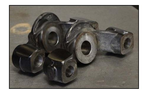
Install the supplied bushings, inner sleeves, and zerk fittings into the new lower control arm, then install the new arm on the vehicle (it make take the use of a dead blow hammer to get the arm into the frame pockets).
