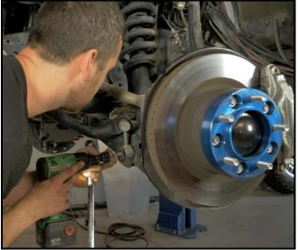
Loosen (do not remove) the two cam bolts that connect the lower control arm to the vehicle using a 24mm wrench or socket.
