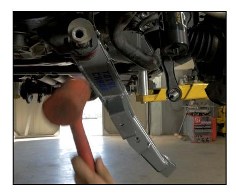
Install the short misalignment in the top of the uniball, the large misalignment into the bottom of the uniball (tapered side down), slide the modified ball joint cradle onto the tapered misalignment, then slide the bolt from the top through all of the pieces then install the washer and tighten the nut using a 5/8" allen wrench and 1 1/8" wrench or socket (110ft/lbs).
