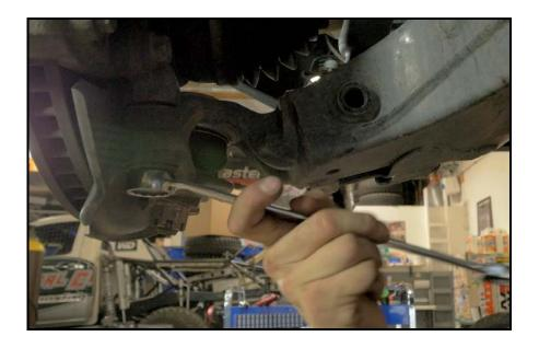
Let the lower control arm pivot down into a vertical position, then remove the two bolts that hold the control arm to the frame, and remove the stock lower control arm from the vehicle.
