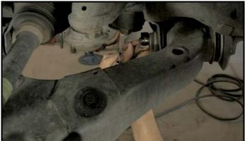
Remove the two bolts that hold the ball joint cradle to the steering knuckle using a 22mm wrench or socket.
