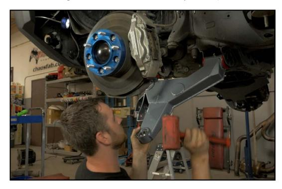
Install the alignment cam bolts that connect the lower control arms to the frame.
