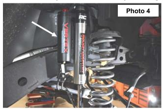
factory hardware using a 18mm wrench after the vehicle is on the ground. Do not install the sway bar link on the sway bar until the sway bar is on the ground.
