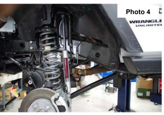
10. The draglink must be adjusted to center the steering wheel **<u>BEFORE</u>** the vehicle is driven. Failure to do so will cause a computer error with the Jeep's traction control system and will result in odd handling and poor performance.
