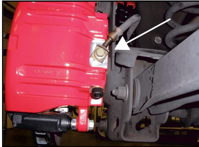
Figure 2: Rear assembly with correct brake hose installation
