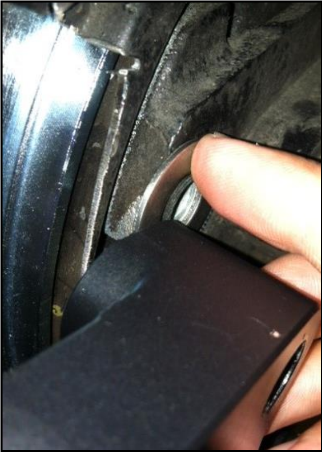
Figure 7: Shim location (between axle housing and bracket)
