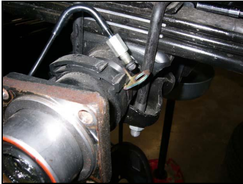
Figure 2: Right (passenger) side hardline retainer position
