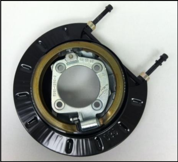
Figure 5: Outboard view of park brake assembly (spacers installed over studs)
