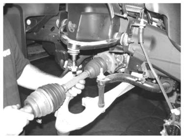
Remove the lower control arms from the frame and retain with the hardware for reinstallation. SEE PHOTO IN NEXT COLUMN.
