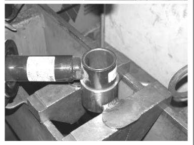
26. Locate Box 3 FTS21042BK which has FT20339 Shock Mount to Arm, FT20323 Shock Extensions, FT20568 Shock Brackets, FT20342 (non auto-ride) or FT20351 (auto-ride) Aluminum Bushings , Hardware Kit FT20295, FT1036 Bushings, and FT148 Sleeves. Using a press, press the bushings and sleeves (with the provided lube) into the shock extension. Insert the Aluminum Bushings into the bottom of the factory shock. SEE PHOTOS IN NEXT COLUMN
