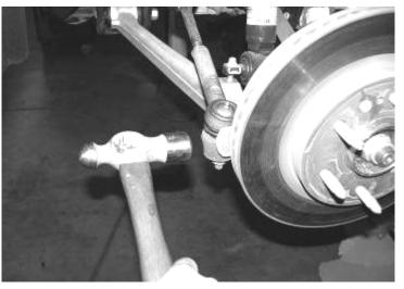
3. Unplug the ABS brake connection from the frame and control arm. Remove the brake hose bracket from the steering knuckle. Remove the brake hose bracket from the strut bucket and save hardware. Remove the caliper from the rotor and secure the brake caliper to the frame out of the way. DO NOT ALLOW THE BRAKE CALIPER TO HANG FROM THE BRAKE LINE HOSE. SEE PHOTO BELOW
