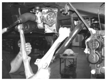
9. Locate, remove, and save the sway bar, discard hardware. SEE PHOTO BELOW
