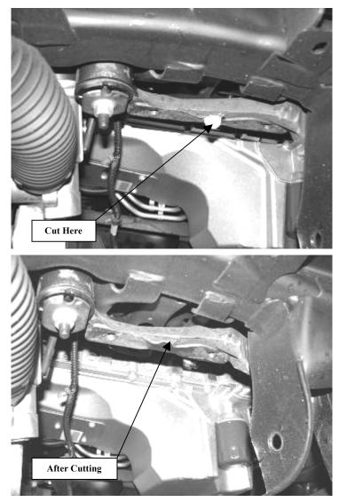
18. Locate FT20347 (driver) & FT20348 (pass) Diff. brackets and the factory diff hardware. Install the brackets to the factory mounts with the taller part of the bracket to the front of the truck with the factory hardware. Torque to 75 ft lbs. SEE PHOTOS BELOW AND IN NEXT COLUMN.
