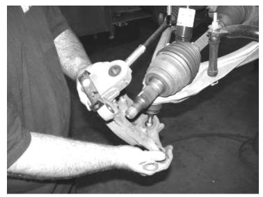
6. Remove the shock assembly and save with the hardware. Remove and discard the factory brake line bracket from the brake hose that attached the hose to the upper control arm. SEE PHOTO BELOW
