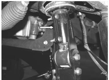
Photo shows new style shock brackets
