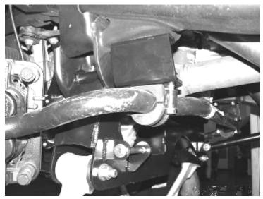
36. Locate FT20602 Sway Bar Mounts and the supplied 18mm x 50mm hardware. Position the Sway Bar Mount so that it is on the bottom of the sway bar with the stop plate on the bottom. Attach with the 18mm hardware and torque to 110 ft lbs. Locate the factory sway bar end links and attach to the new mount and the lower control arm. SEE PHOTOS BELOW.
