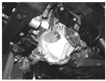
20. Locate and install FT20283 rear crossmember into the factory lower control arm pockets using the stock hardware and leave loose at this time. (CHECK THE CLEARANCE OF THE DIFF TO CROSSMEMBER WHERE IT WAS SANDED DOWN IN STEP #18 FOR ADAQUATE CLEARANCE TO THE FRAME AND CROSSMEMBER ) SEE PHOTO ON NEXT PAGE.
