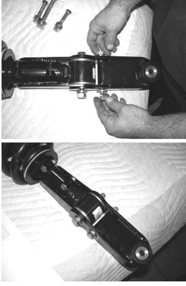
Locate the factory upper shock hardware. Install the shock into the factory shock bucket and leave loose. SEE PHOTOS BELOW AND ON NEXT PAGE.
