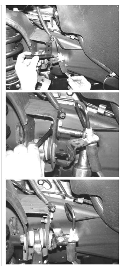
38. Re-route the brake hose and the ABS Line to the steering knuckle using the adel clamp to the back of the steering knuckle and attach with ¼" x 3/4" bolt and washer. Torque to 10 ft LBS. Route the ABS line next to the brake hose. Re-connect the ABS line to the harness in the wheel well. Using provided plastic tyraps secure line to the hose and away from the tire and wheel. SEE PHOTO BELOW
