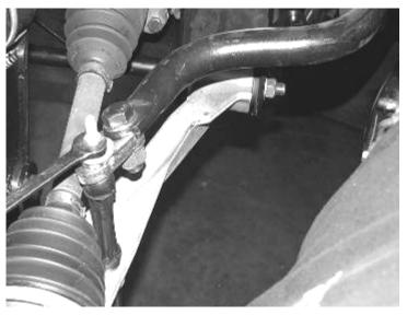
37. Locate FT20313 (drv.) FT20314 (pass) Brake Line Bracket and ¼" x ¾" hardware. Position the new bracket into the factory brake line bracket location and attach with the factory hardware and the ¼" hardware. Attach the factory brake line bracket to the new Fabtech bracket. Carefully bend the hard brake line and attach with the supplied ¼" hardware. Torque to 10 ft LBS. SEE PHOTOS IN NEXT COLUMN.
