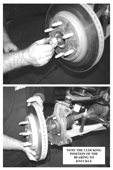
5. Remove the upper and lower ball joint nuts. Disconnect the upper and lower ball joints from the steering knuckle by striking the knuckle with a large hammer next to each ball joint on the knuckle to dislodge the ball joints. Use care not to hit the ball joints when removing. Save nuts and discard knuckle. SEE PHOTO BELOW
