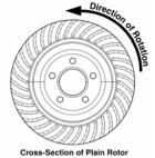
the rotor hat area with either an arrow, or an "L" for left, or an "R" for right, or both. "L" or left, always indicates the driver's side of US spec vehicles.
